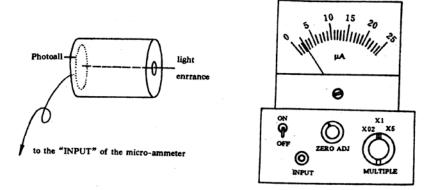
Fig. 2 Light intensity detector
