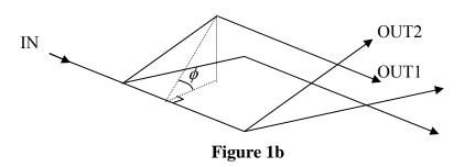
**Physical situation** We consider the situation of the famous neutron-interferometer experiment by Collela, Overhauser and Werner, but idealize the set-up inasmuch as we shall assume perfect beam splitters and mirrors within the interferometer. The experiment studies the effect of the gravitational pull on the de Broglie waves of neutrons.
