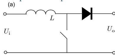
(b) Now, the key is switched on and off periodically; each time, the key is kept closed for time interval  $\tau_c$  and open — also for  $\tau_c$ . Find the average output current.
