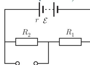
**idea 11:** Sometimes it is convenient to deal with constant current sources — instead of batteries (and sometimes, a current source is already present). A battery with electromotive force  $\mathcal{E}$  and internal resistance  $r$  is equivalent to a constant current source with  $I = \mathcal{E}/r$  which is connected parallel to the shunt resistance  $r$ <sup>11</sup>.
