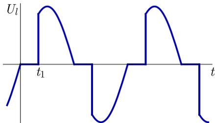
(c) The voltage  $U_l$  on the lamp follows the plot above. Let's assume that the assumption of part i) and the inequality of part ii) hold. Find the time  $t_0$  during which the voltage on the lamp is zero.
