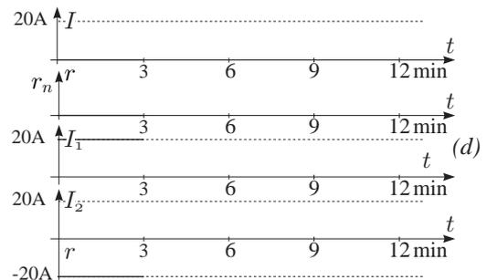
(d) Suppose the magnet is operated in a persistent mode with a persistent current of  $20 \text{ A}$  [ $t = 0$  to  $t = 3 \text{ min}$ . See Fig. (e)]. How would you change it to a persistent mode with a current of  $30 \text{ A}$ ? plot your answer in Fig. (e).
