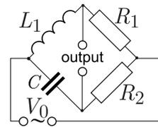
**pr 109.** In the circuit shown in the figure, the sinusoidal input voltage has a fixed amplitude  $V_0$  and frequency  $f$ . What is the maximal amplitude of the output voltage, and for which values of the variable resistances  $R_1, R_2$ , and  $R_3$  is the maximal amplitude achieved?
