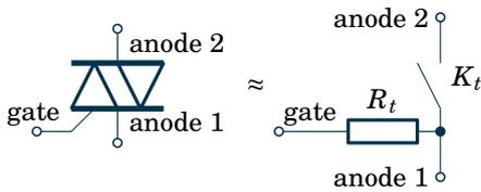
The switch  $K_t$  is open as long as the current through the triac's gate stays under the threshold current  $I_t$ ; closes when the threshold current is applied (in either direction) and stays closed while a current is flowing through the switch  $K_t$  (the gate current is irrelevant until the switch opens again).
