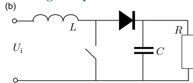
(c) Now, circuit (a) is substituted by circuit (b); the switch is switched on and off as in part ii. What will be the voltage on the load  $R$ , when a stationary working regime has been reached? You may assume that  $\tau_c \ll RC$ , i.e. the voltage variation on the load (and capacitor) is negligible during the whole period (i.e. the charge on the capacitor has no time to change significantly).
