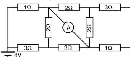
**pr 37.** The drawing below depicts octahedron made from wire; the number near to each edge shows the resistance of the corresponding wire in ohms. The resistance of the wires connecting the ammeters are negligibly small. Find the readings of the ammeters.
