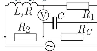
**pr 95.** Below a circuit is given which makes it possible to adjust the phase of a voltage signal. Show that if the output current is negligibly small, its voltage amplitude will be the same as at the input leads, but with a different phase. Find the phase shift.
