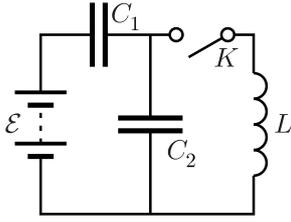
One way of solving this problem is using the idea 35, together with the energy conservation law. The second way is to study the voltage (and current) oscillations in the circuit. LC-circuit oscillations will be studied later in more details; here it is enough to formulate one more “fact”.
