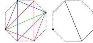
For a precise calculation, consider this side-less octagon as the octagon of the problem 48, which has additionally negative resistances  $-R$  connected parallel to the sides (idea 23). Further, apply the generalized idea 9: represent the octagon of the problem 48 as a  $Y$ -connection of 8 identical resistors. Finally, calculate the resistance using the idea 1.
