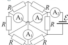
**pr 36.** Find the reading of the ammeter in the circuit below.
