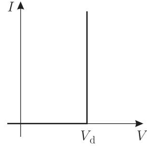
**pr 59.** A capacitor is charged by connecting it to a series connection of a battery of electromotive force  $\mathcal{E}$ , inductor of inductance  $L$ , and a diode. For the  $V$ - $I$  dependence of the diode use the graph of the previous problem; internal resistance of the battery is negligible. To which voltage the capacitor will be charged, assuming that  $\mathcal{E} > V_d$ ?
