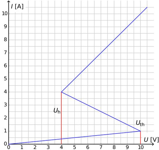
(a) Using the graph, determine the resistance  $R_{on}$  of the element  $X$  on the upper branch of the  $I - V$  characteristics, and  $R_{off}$  on the lower branch, respectively. The middle branch is described by the equation  $I = I_0 - \frac{U}{R_{int}}$ . Find the values of the parameters  $I_0$  and  $R_{int}$ .
