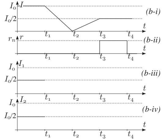
(b) Suppose the power switch  $K$  is turned on at time  $t = 0$  when  $r = 0$ ,  $I_1 = 0$  and  $R = 7.5 \Omega$ , and the total current  $I$  is  $0.5 \text{ A}$ . With  $K$  kept closed, the resistance  $r$  of the superconducting switch is varied in the way shown in Fig. (c)-ii. Plot the corresponding time dependences of  $I$ ,  $I_1$  and  $I_2$  in Figs. (c)-i, (c)-iii and (c)-iv respectively.
