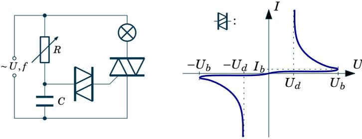
A diac  $\overline{\overline{\nabla}}$  is a component whose behaviour is determined by the voltage-current diagram shown above. A triac  $\overline{\overline{\nabla}}$ , on the other hand, can be thought of as a switch controlled by current — look at the following equivalent schematics.
