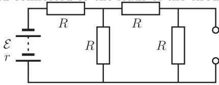
**pr 31.** Find the current through the diode in the circuit given below; for the diode, use the  $I(V)$  dependence from the problem 24.
