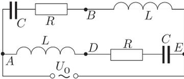
**pr 98.** A circuit consists of two identical inductances, two identical capacitors, and one resistor, see figure. The applied voltage is  $U_0 = 10\text{ V}$ , and the total current at the input leads is  $I_0 = 1\text{ A}$ ; the voltage measured at the left capacitor is  $10\text{ V}$ , and  $10\text{ V}$  is also measured at the left inductance. What is the active power dissipated in this circuit and what is the resistance of the resistor?
