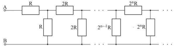
**pr 52.** Find the voltage between the terminals  $A$  and  $B$  for the infinite chain shown below.
