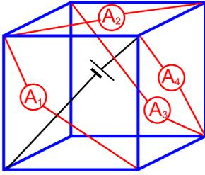
**pr 43.** Four ammeters with identical internal resistances  $r$  and a resistor of resistance  $R$  are connected to a current source as shown in figure. It is known that the reading of the ammeter  $A_1$  is  $I_1 = 3\text{ A}$  and the reading of the ammeter  $A_2$  is  $I_2 = 5\text{ A}$ . Determine the ratio of the resistances  $R/r$ .
