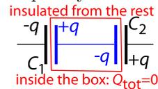
**pr 60.** Show that the series connection of capacitors of capacitance  $C_1, C_2, \dots, C_n$  has net capacitance  $C = (C_1^{-1} + C_2^{-1} + \dots + C_n^{-1})^{-1}$ .
