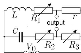
**pr 110.** Find such frequencies of the input voltage  $\omega$  for which the circuit shown below has zero impedance.
