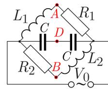
**pr 108.** For the circuit shown below, the frequency of the sinusoidal input voltage is unknown; given the capacitance  $C$ , inductance  $L$ , resistances  $R_1, R_2$ , amplitude of the input voltage  $V_0$ , and the phase shift  $\varphi$  between the inductor current and input voltage, what is the phase shift between the capacitor voltage and output voltage?
