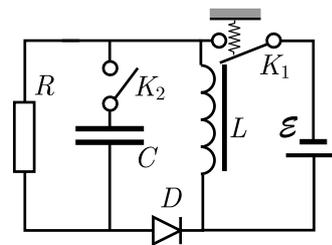
An electromagnetic switch  $K_1$  connects a battery of electromotive force  $\mathcal{E}$  to an inductor of inductance  $L$ : it is closed if there is no current in the inductor (a spring keeps it closed), but if the inductor current reaches a critical value  $I_0$ , magnetic field created by the inductor pulls it open. Due to inertia, once the key is open, it takes a certain time  $\tau_K$  to close again even if the current falls to zero.
