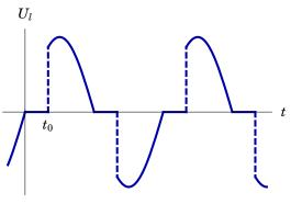
iii) (2 points) The voltage  $U_l$  on the lamp follows the plot above. Let's assume that the assumption of part i) and the inequality of part ii) hold. Find the time  $t_0$  during which the voltage on the lamp is zero.
