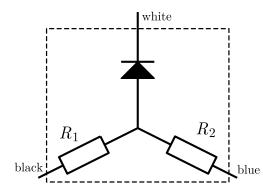
**iii)** From the current measurements we can already calculate 4 datapoints for the current voltage curve of the diode. We obtain additional two datapoints by measuring the current while the resistors inside the black box are connected in parallel.
