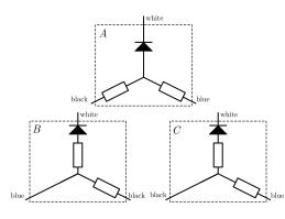
We can deduce the correct schematics of the black box from these measurements, but there are more straightforward ways to test these options. One is to measure the voltage  $U_1$  between "black" and "blue", while connecting the battery between "black" and "white". Secondly measure the voltage  $U_2$  between "blue" and "black", while connecting the battery between "blue" and "white".
