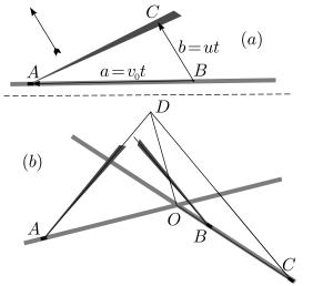
1) Let us draw from an arbitrary point B on the road a line parallel to the direction of the wind, and let it intersect the smoke trail at point C. Then, the smoke emitted by the tractor at Bhas travelled the distance |BC| = ut, where u is the wind speed. Tractor itself has travelled the distance  $|AB| = v_0 t$ . So, we can measure the distances |AB| and |BC from the figure and calculate
