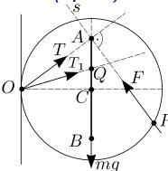
The friction force  $F_f$  cannot exceed  $\mu N$ , where N is the normal force. Hence, the resultant vector  $\vec{T}$  of those two forces must point to some point Q on the segment AB, the length of which is  $2\mu R$ , and R stands for the radius of the ball (so that  $AC = \mu R$ , where C is the ball's center).
