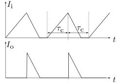
The average output current J is the surface area under one period of the graph, divided by the period length. So,  $J = \frac{1}{2}I_{\max}\tau_1/(2\tau_c)$ , where  $\tau = \tau_c \frac{U_i}{U_0 - U_i}$  is the length of a time segment when  $I_o > 0$ . So,
