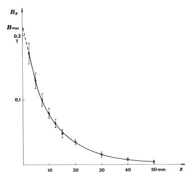
Fig. 18 Magnetic induction vs. distance
