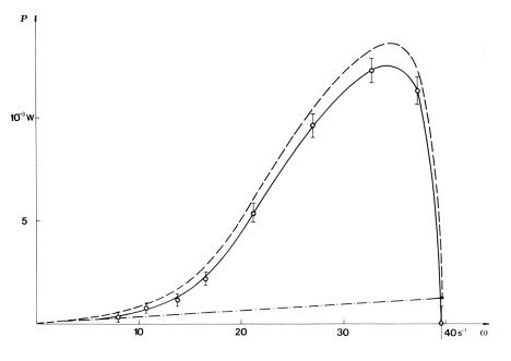
Fig. 13 Net power (full line), power loses (dashed and dotted line) and total power (dashed line) vs. angular velocity
