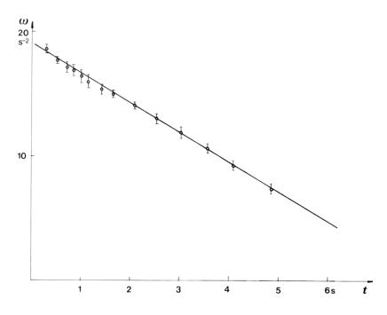
Fig. 14 Angular velocity vs. time during deceleration
