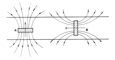
Fig. 15 A typical implementation of the magnets in the block
