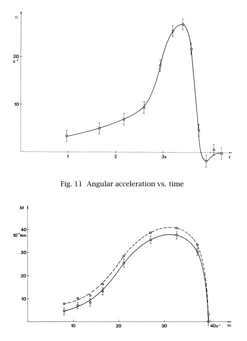
Fig. 12 Net torque (full line) and total torque (dashed line) vs. angular velocity
