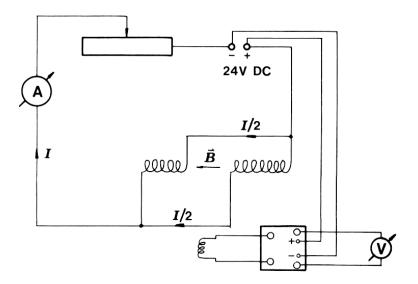
Fig. 17 Calibration of the measuring system
