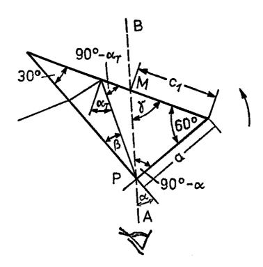
Draw a straight line A - B on a sheet of paper and let this be your line of sight. Place the prism with its rectangular edge facing you onto the line (at point P on the line). Now turn the prism in the direction of the arrow until the dark edge of total reflection which can be seen in the short face of the prism coincides with the  $90^{\circ}$  edge of the prism. Mark a point M and measure the length  $c_1$ . Measure also the length of the short face of the prism.
