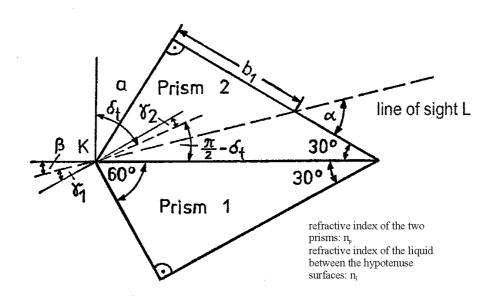
If the refractive index of the prism is known (see part a) the refractive index of the liquid may be calculated as follows:
