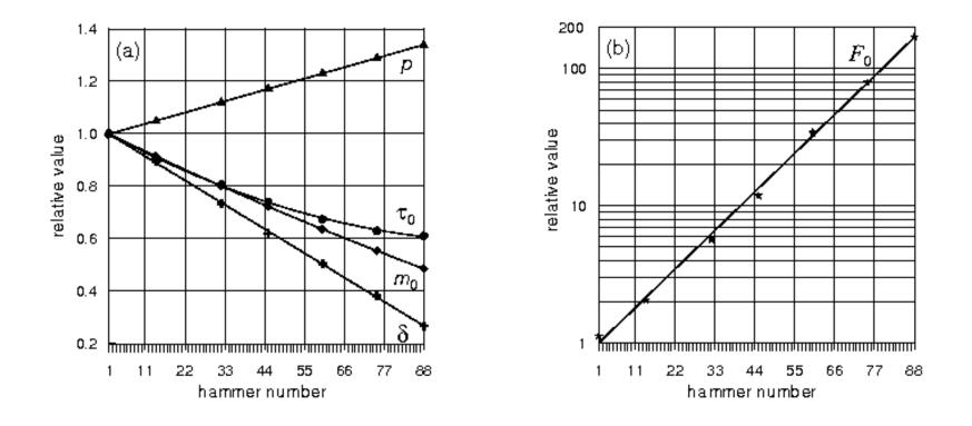
Parameters of hammer n=1  $p = 3.72; \tau_0 = 2.7 \text{ } \mu \text{s}; m_0 = 11 \text{ } \text{g}; \delta = 1 - \epsilon = 0.011; F_0 = 16440 \text{ N/mm}^p$
