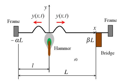
"When the hammer has less mass than the string, it will most likely be thrown clear of the string by the first reflected pulse."
