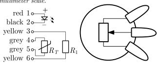
The schematic and connections of the circuit board (left) and the potentiometer (right) are in the figure. The resistor  $R_1$  may be used for heating the board near the LED. The temperature sensor (thermistor)  $R_T$  is another resistor whose resistance depends strongly on the absolute temperature T:
