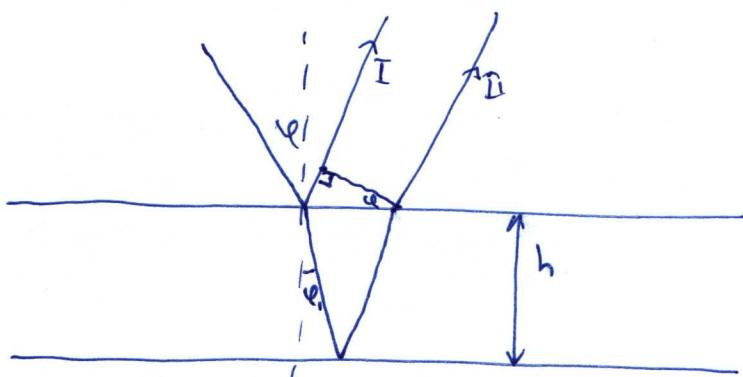
Difference of optical length between beams I and II is
