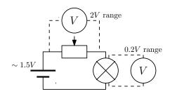
The resistance of the rheostat can be measured directly, or using current/voltage measurements,  $R_r = 25.3 \,\Omega$  $(0.1 \, \mathrm{pts})$
