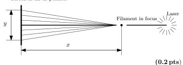
We focus the laser to the filament, holding the screen close to the filament during the adjustments helps focusing. For the measurements we place the screen perpendicular to the beam and reasonably far back  $(x \ge 50 \,\mathrm{cm})$  to get the maxima spaced out.  $(0.2 \, \mathrm{pts})$
