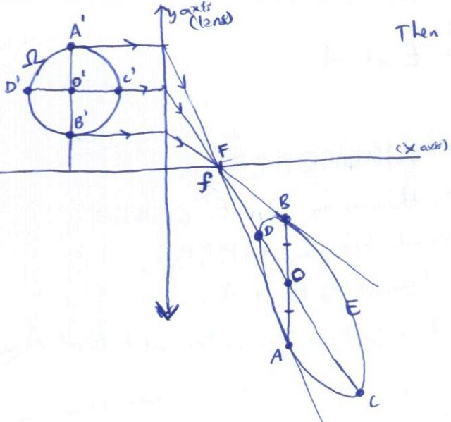
Then it is easy to see that if  $A'$ ,  $C'$ ,  $B'$ ,  $D'$  and  $O'$  are the north, east, south, west and center of  $\Omega$ , and  $F$  is point of the focus opposite  $\Omega$ , then by ray tracing, size  $A, O, B$  are same distance from the lens and  $O'$  is midpoint of  $A'B'$ . ( $AOB \parallel$  rays) their images thus,  $A, O, B$  are all same distance from the lens and  $O$  is midpoint of  $AB$  (equal magnification).
