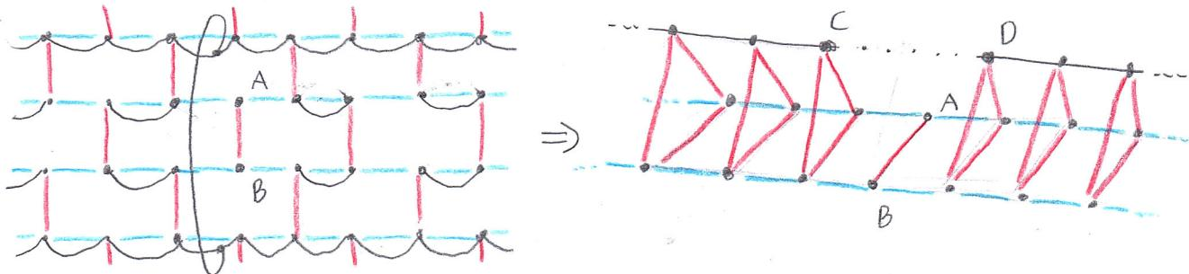
Points C and D are equipotential because of the symmetry of the circuit (the current is driven into lead A and out from lead B), so the wire between them can be cut off.
