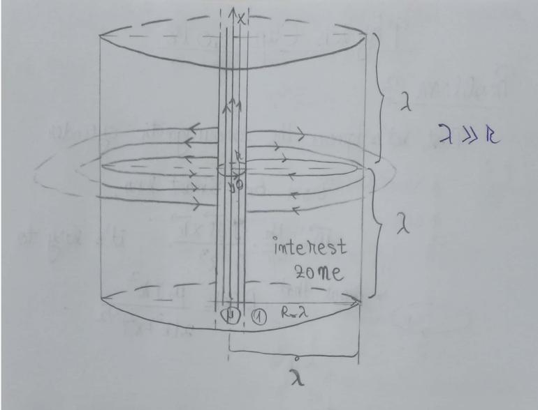
The infinite ferromagnetic cylinder will channel the magnetic field lines like above. The magnetic field lines like above the magnetic field in Nide the cylinder will be much stronger then the outside field.
