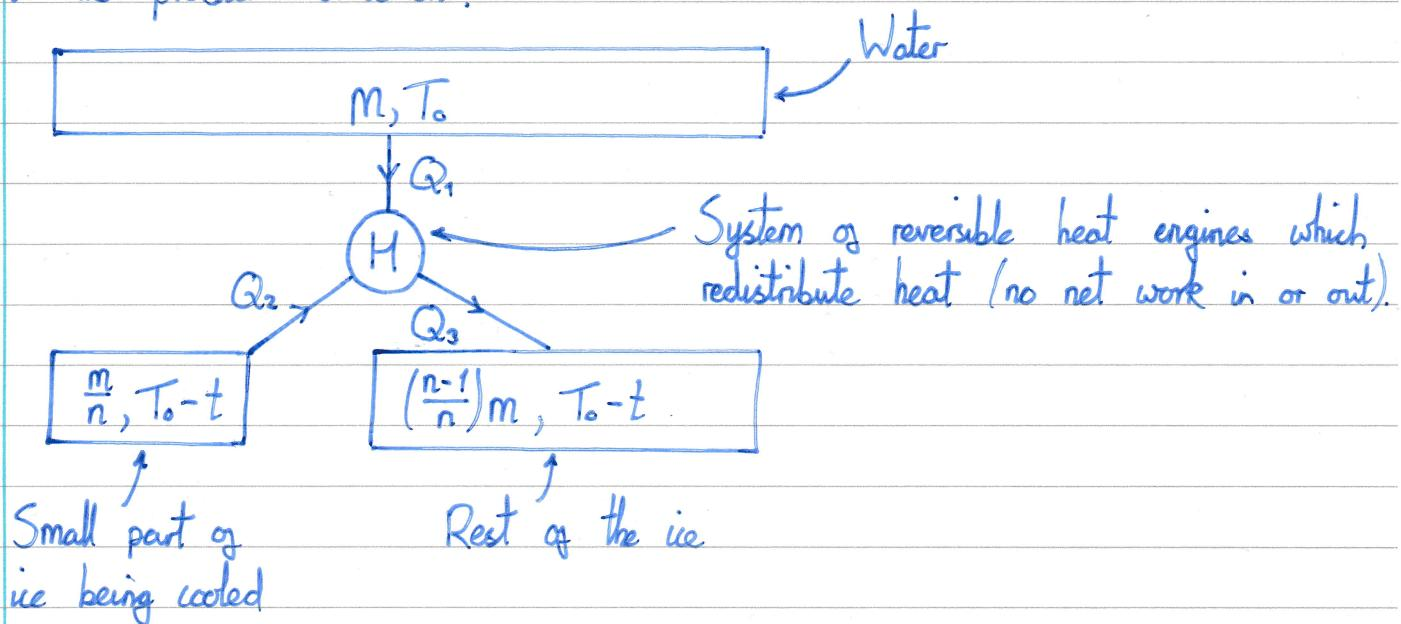
In the initial state, the whole system except the part being cooled must have the same temperature because any temperature difference could be used to power a heat engine and achieve further cooling.
