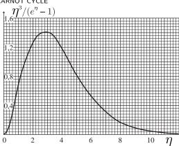
In many applications it is necessary to keep the satellite as cool as possible. To cool the satellite, engineers use a reflective coating that reflects light above a cut-off frequency but does not prevent heat radiation at lower frequency from escaping. Assume that this (sharp) cut-off frequency corresponds to  $hf/k = 1200 \,\mathrm{K}.$
