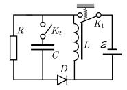
An electromagnetic switch  $K_1$  connects a battery of electromotive force  $\mathcal{E}$  to an inductor of inductance L: it is closed if there is no current in the inductor (a spring keeps it closed), but if the inductor current reaches a critical value  $I_0$ , magnetic field created by the inductor pulls it open. Due to inertia, once the key is open, it takes a certain time  $\tau_K$  to close again even if the current falls to zero.
