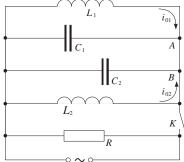
(a) Find the ratio of frequency  $\nu_M/\Delta\nu$ , where  $\nu_m$  is the frequency for which the active power in circuit has the maximum value  $P_m$ , and the frequency difference  $\Delta\nu = \nu_+ - \nu_-$ , where  $\nu_+$  and  $\nu_-$  are the frequencies for which the active power in the circuit is half of the maximum power  $P = \frac{1}{2}P_m$ .
