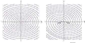
$-CV_d < q < CV_d$ ;  $\Delta q = -4CV_d$ ,  $t = N\pi\sqrt{LC}$ ,  $N = \left\lfloor \frac{|q_0| - CV_d}{2CV_d} \right\rfloor$ ; a mass-spring system where the mass is subject to a dry friction force.
