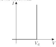
**pr 59.** A capacitor is charged by connecting it to a series connection of a battery of electromotive force  $\mathcal{E}$ , inductor of inductance L, and a diode. For the V-I dependence of the diode use the graph of the previous problem; internal resistance of the battery is negligible. To which voltage the capacitor will be charged, assuming that  $\mathcal{E} > V_d$ ?
