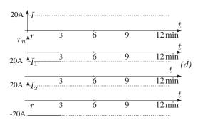
(d) Suppose the magnet is operated in a persistent mode with a persistent current of 20 A [t = 0 to t = 3 min. See Fig. (e)]. How would you change it to a persistent mode with a current of 30 A? plot your answer in Fig. (e).
