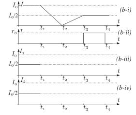
(b) Suppose the power switch K is turned on at time t = 0when r = 0,  $I_1 = 0$  and  $R = 7.5 \Omega$ , and the total current I is 0.5 A. With K kept closed, the resistance r of the superconducting switch is varied in he way shown in Fig. (c)-ii. Plot the corresponding time dependences of I,  $I_1$  and  $I_2$  in Figs. (c)-i, (c)-iii and (c)-iv respectively.
