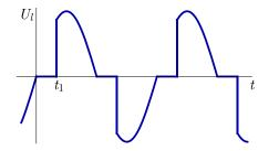
(c) The voltage  $U_l$  on the lamp follows the plot above. Let's assume that the assumption of part i) and the inequality of part ii) hold. Find the time  $t_0$  during which the voltage on the lamp is zero.
