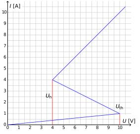
(a) Using the graph, determine the resistance  $R_{\rm on}$  of the element X on the upper branch of the I - V characteristics, and  $R_{\rm off}$  on the lower branch, respectively. The middle branch is described by the equation  $I = I_0 - \frac{U}{R_{\rm int}}$ . Find the values of the parameters  $I_0$  and  $R_{\rm int}$ .
