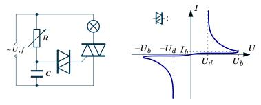
A diac  $\overleftrightarrow$  is a component whose behaviour is determined by the voltage-current diagram shown above. A triac  $\overleftrightarrow$ , on the other hand, can be thought of as a switch controlled by current — look at the following equivalent schematics.
