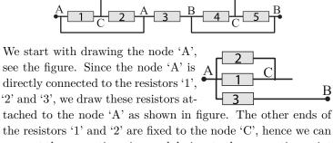
the resistors '1' and '2' are fixed to the node 'C', hence we can connect the respective wires and designate the connection point by 'C'. Further, the other end of the resistor '3' is connected to the node 'B', so we draw a wire and mark its end with 'B'. Now, by noticing that the resistors '4' and '5' connect the nodes 'B' and 'C', it is easy to complete the circuit.
