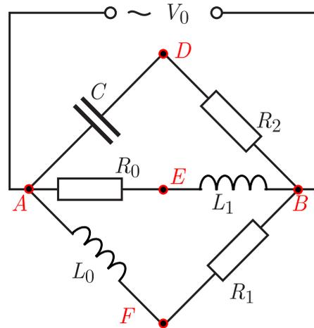
i) (2 points) Draw a phasor diagram for this circuit showing the voltage vectors between the following nodes:  $V_{AD}$ ,  $V_{DB}$ ,  $V_{AB}$ ,  $V_{AE}$ ,  $V_{EB}$ ,  $V_{AF}$ , and  $V_{FB}$ .
