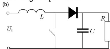
iii) (2 pt) Now, circuit (a) is substituted by circuit (b); the switch is switched on and off as in part ii. What will be the voltage on the load  $R$ , when a stationary working regime has been reached? You may assume that  $\tau_c \ll RC$ , i.e. the voltage variation on the load (and capacitor) is negligible during the whole period (i.e. the charge on the capacitor has no time to change significantly).
