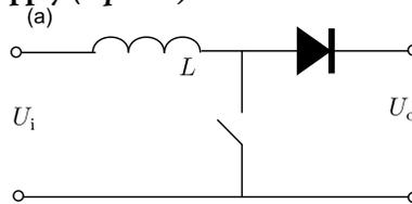
i) (2 pt) Consider the circuit given in Fig (a), where the diode can be assumed to be ideal (i.e. having zero resistance for forward current and infinite resistance for reverse current). The key is switched on for a time  $\tau_c$  and then switched off, again. The input and output voltages are during the whole process constant and equal to  $U_i$  and  $U_o$ , respectively ( $2U_i < U_o$ ). Plot the graphs of input and output currents as functions of time.
