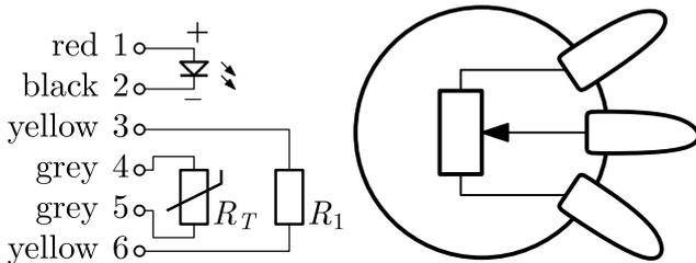
The schematic and connections of the circuit board (left) and the potentiometer (right) are in the figure. The resistor  $R_1$  may be used for heating the board near the LED. The temperature sensor (thermistor)  $R_T$  is another resistor whose resistance depends strongly on the absolute temperature  $T$ :
