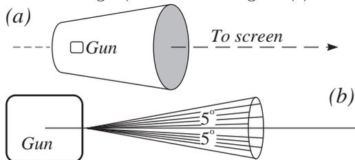
The electron beam emerges from the anode of the electron gun on the axis, but with a divergence of up to  $5^\circ$  from the axis, as illustrated in figure (b). In general a diffuse spot is produced on the screen, but for certain values of the magnetic field a sharply focused spot is obtained.
