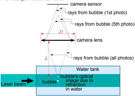
In the figure below, the taken photos are placed side by side and indicated by numbers 1-5. **Task:** calculate the diameter of the gas bubble.
