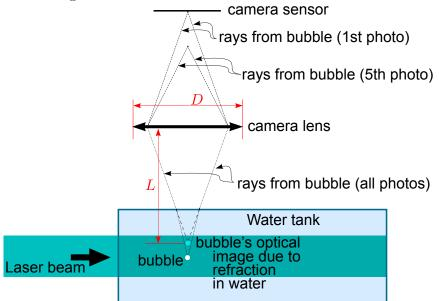
In the figure below, the taken photos are placed side by side and indicated by numbers 1-5. **Task:** calculate the diameter of the gas bubble.
