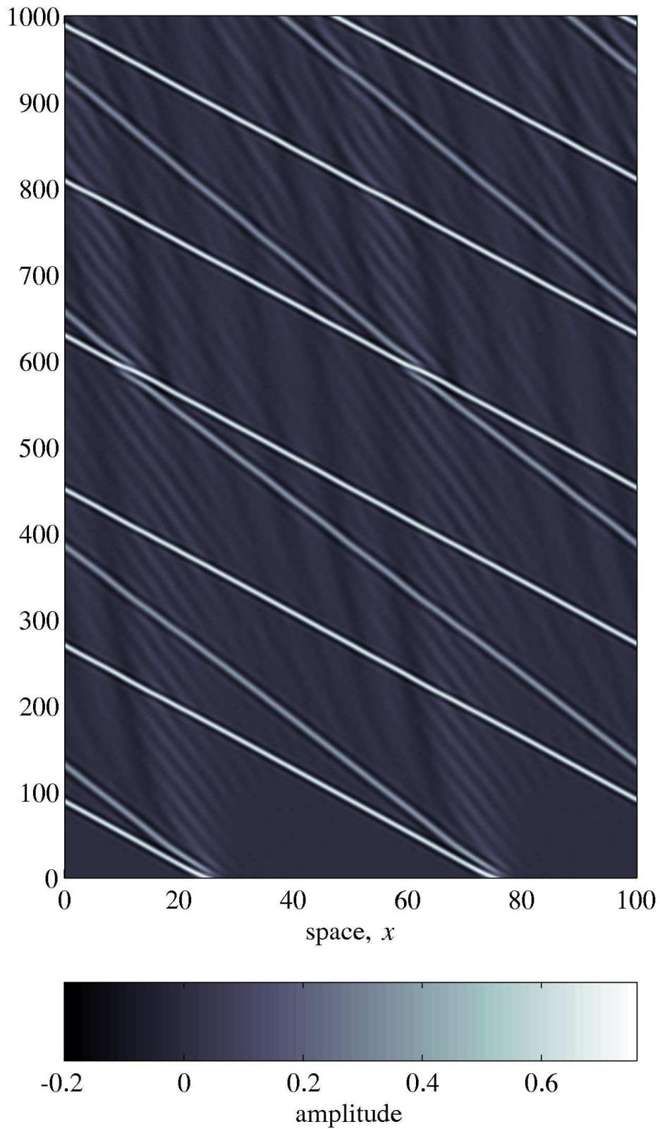
Fig. 16. Two solitary waves. Pseudocolor plot over two space periods in the case of  $d_l = 1.2$ ,  $b_l = 2.0$ ,  $A = 0.71$  and  $0 < t < 1000$ .
