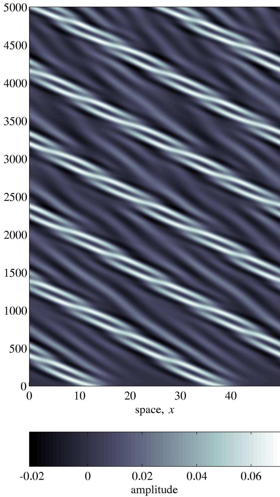
Fig. 8. “Plaited” solitons. Pseudocolor plot over two space periods in the case of  $d_l = 1.6$ ,  $b_l = 2.0$ ,  $A = 0.063$  and  $0 < t < 5000$ .
