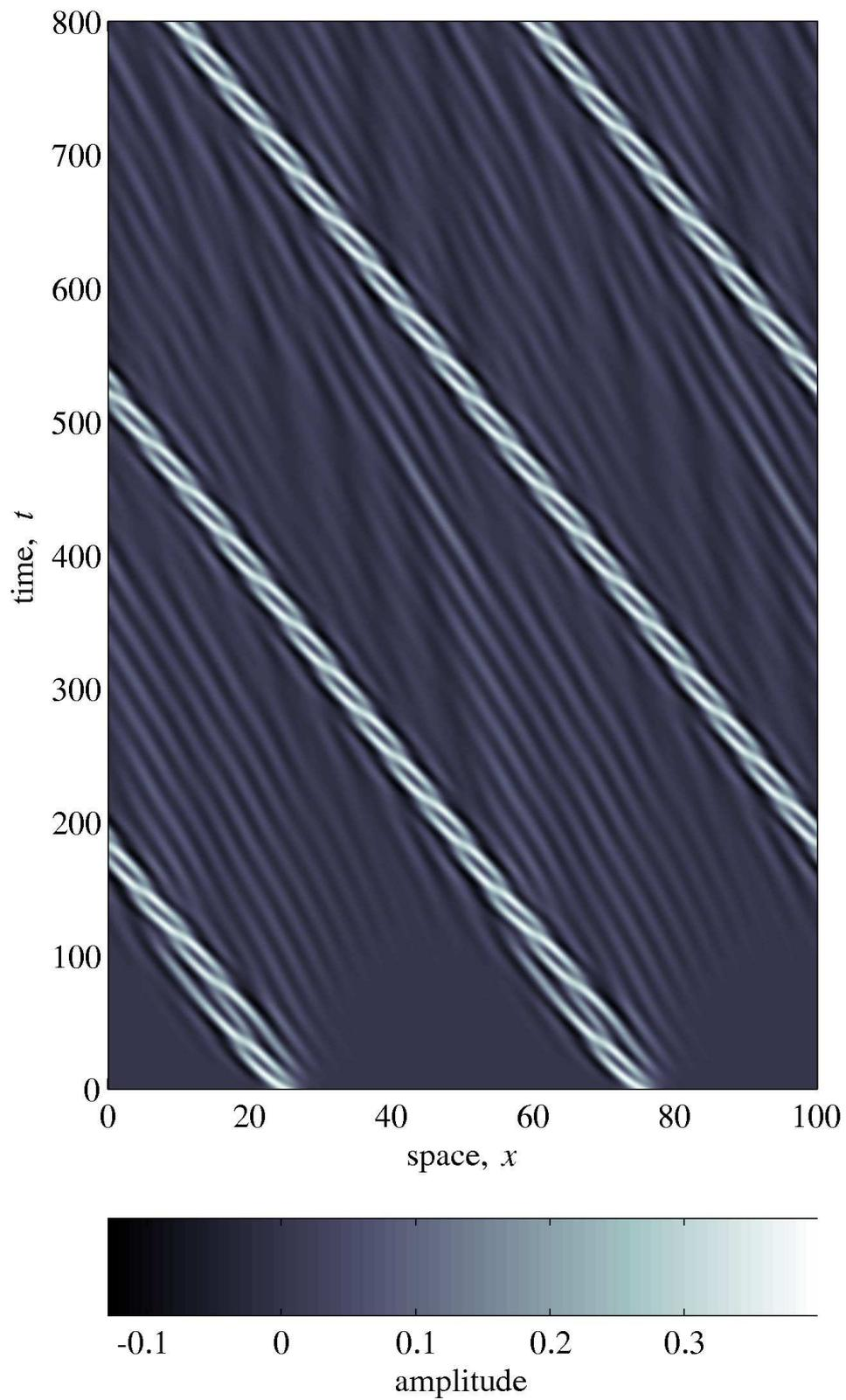
Fig. 10. "Plaited" solitons. Pseudocolor plot over two space periods in the case of  $d_l = 1.2$ ,  $b_l = 2.0$ ,  $A = 0.37$  and  $0 < t < 800$ .
