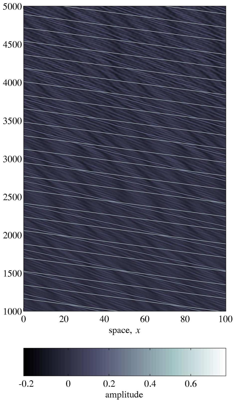
Fig. 17. Two solitary waves. Pseudocolor plot over two space periods in the case of  $d_l = 1.2$ ,  $b_l = 2.0$ ,  $A = 0.71$  and  $1000 < t < 5000$ .
