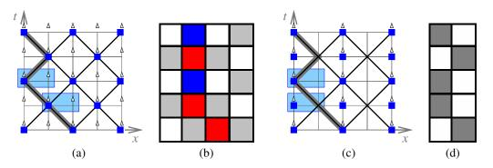
Figure 1.9: **Two more rendering options for 1D diffusion** This figure is similar to Fig. 1.8, but depicts two more rendering options. (a) and (b) show the space-time diagram and results for a rule called rgb \_block that renders 1 and r to red[0] and blue[1] . (c) and (d) show grayscale rendering with output signals that are on the same sparse sublattice (spacing 2) of the grid that the signals are on.
