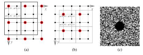
Figure 1.14: The Margolus neighborhood HPP BPCA (a) and (b) depict the lattices employed in the BPCA version of HPP and the partitionings imposed by the rule's lattice. The signal lattice is allocated on the grid and depicted using small squares while the rule's lattice has a spacing of (2, 2) and is depicted using large red circles. (c) shows the rendering results when the signal cosets are rendered directly to an image.
