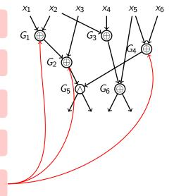
by a short case analysis it is possible to show that this way one can always eliminate 3 gates; since we can make n - o(n) such substitutions a lower bound 3n - o(n) follows
