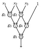
• Shannon counting argument: count how many different Boolean functions in *n* variables can be computed by circuits with *t* gates and compare this number with the total number  $2^{2^n}$  of all Boolean functions.
